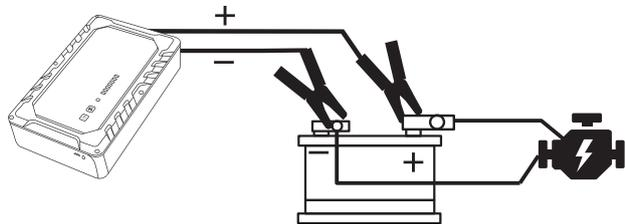
Connect the red clamp (+) to the battery's (+) terminal.
