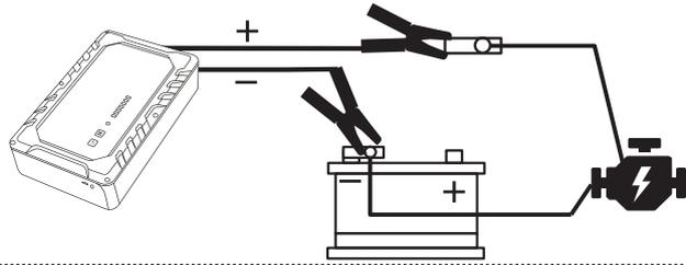
Unplug the (+) connector from your battery's terminal and connect the STARTRONIC's red clamp (+) to it. Connect the black clamp (-) to the (-) terminal on the battery.
