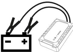
Connect the STARTRONIC to a substitute 12V battery and press the on/off button to start. *(Full charge will take approximately 2 minutes.)*
