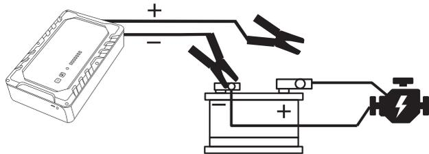
Remove the red clamp (+) from the battery's (+) terminal.
