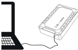
The STARTRONIC can be charged via its micro USB port (2) with any device equipped with a USB port 5V 2A. USB charging cable not supplied. *(Full charge will take approximately 15 minutes.)*
